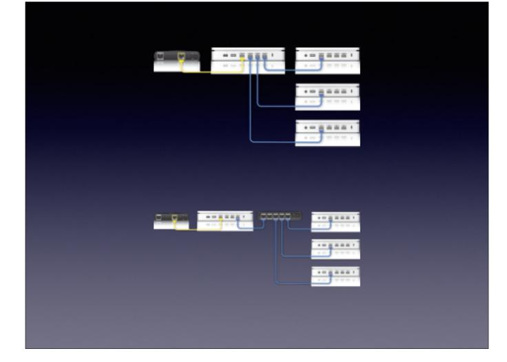
Alternately, you can connect multiple access points together with wired Ethernet. In this case, they'll all work together to extend your network without consuming extra wireless bandwidth for communicating with each other. You run into a different problem here in that the APs all need to avoid each other's frequencies, but that's also a problem with wireless extension. This is the best way to do network extension, but it's also not necessarily the most convenient, because you gotta run wires.
