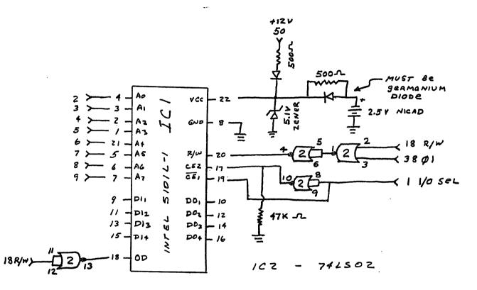
The above diagram depicts only one half of the memory. ICl is a 256 X 4 RAM and it takes two to give a 256 byte memory. It is essential to use the Intel 5101L-1 chip or an exact equivalent.\*
