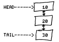
The values of HEAD and TAIL directly index the list. The lines between the boxes represent implied links which connect each entry with the next entry. The between node links are implied because we know that in order to so down from the current entry you add one. To so up you subtract one. The numbers inside the squares are the values of the array at that node.
