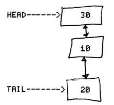
There is no way to print the contents in ascending order. What is needed is a redesign of the links between each node. By making the UP/DOWN links explicit we can provide a path by which the contents of the array can be accessed in order. This is called the doubly linked list structure. The program on the next page uses this structure to keep track of the 'N' largest numbers in an input stream.
