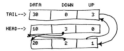
Notice that the down pointer of the tail is zero and the up pointer of the head is also zero. A zero pointer means there is no where to so.
